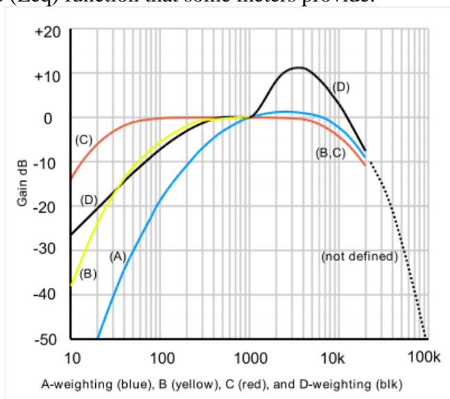
**Figure 8. Comparison of sound measurement weighting filters**
